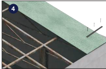
Secure the lower end by screwing a termination bar.
